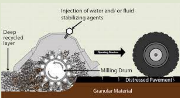
Pulverizing Existing Roadway
