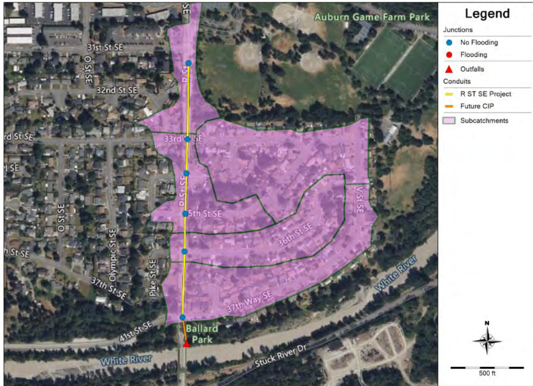
Figure B-7. Plan View of R Street SE Widening and Future CIP (R Subbasin Model, 25-year storm flows [10/20/2003])
