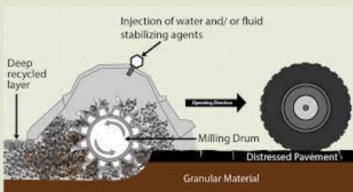
Pulverizing Existing Roadway
