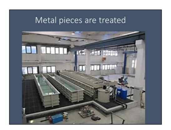
Metal parts are dipped into different solutions...often acidic solutions with dissolved metals...those treatments are done to make the part tougher, stronger, more weather resistant.
