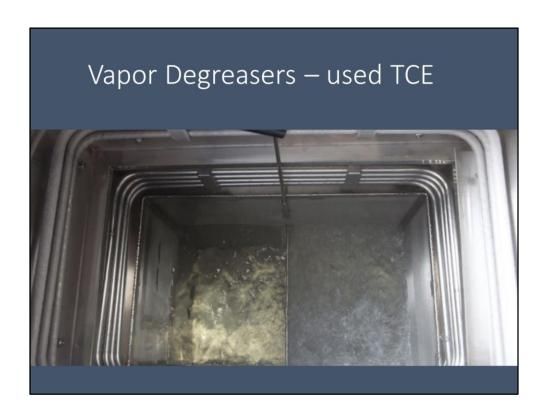
After machining, the part is slippery, so it needs to be cleaned. The cleaner of choice (not just at Boeing Auburn – but EVERYWHERE) until about 1992 was vapor degreasing with TCE.
